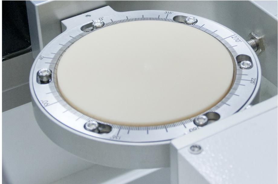
If not using a new blank workpiece, ensure that the workpiece is positioned and oriented correctly so that the milling is made on blank space of the workpiece.
