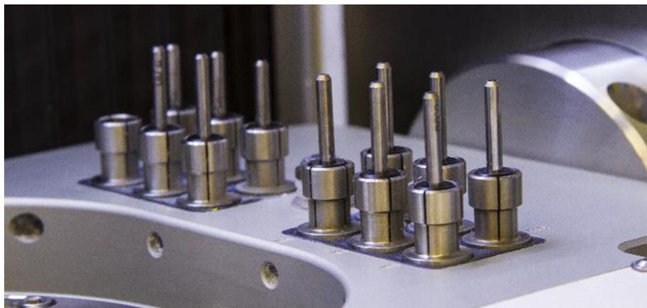
5. Make sure you do not strike or damage the tools during insertion
