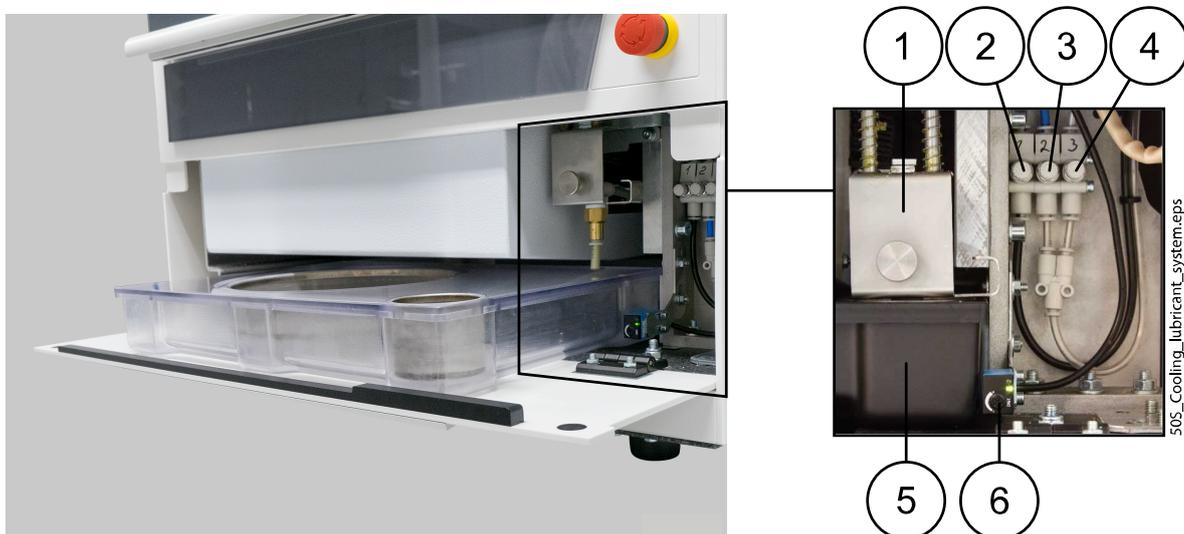
1. Extraction device (manually extending and retracting)
