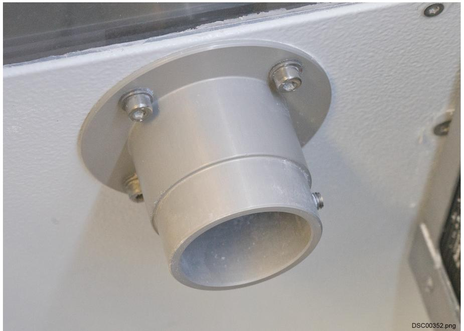
3. Close the extraction nozzle by placing the protective cap onto it.
