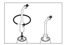
> Insert the torque wrench into the instrument holder as shown.
