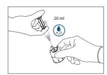
> Use a disposable 20 ml syringe to aspirate and inject tap water for minimum 1 minute (temperature < 35 °C) into the hose and the male coupling of the Irrigation Circuit Cleaning Kit.
