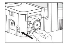
> Re-position the plastic cover on the peristaltic pump.
