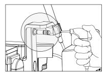
> Place the new o-ring in its seat being careful not to damage it by drilling it with the removal tool and dilating it as little as possible during insertion.
