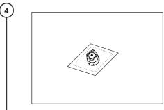
> Seal the combination wrench individually inside a disposable pouch for sterilization.
