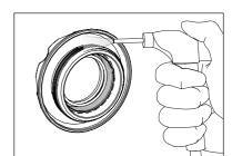
> Place the new o-ring in its seat dilating it as little as possible during insertion.
