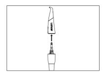
If the Lunos® Perio Tip has been used, remove the subgingival perio tip using the combination wrench supplied and then proceed with the disposal (Chapter 11 on page 91);
