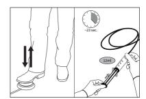
Directly continue with disinfection of the polisher side circuit from step 1 (see Chapter 7.4 on page 48). Before starting to work again, the disinfectant has to be removed from the system according to the rinsing procedure (see Chapter 7.5.3 on page 53).
