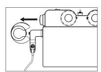
> Remove the Lunos® nozzle with a slight twist movement;
