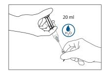
aspirate and inject tap water for minimum 1 minute (temperature < 35 °C) into instruments torque wrench hard-to-reach areas (through holes, internal cavities, grooves and crevices).
