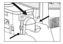
> Disconnect the two silicon tubes of the peristaltic pump from their respective couplings, which are positioned beneath the pump;
