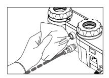
> Screw the male coupling supplied with the Irrigation circuit cleaning kit into the housing until it reaches the stop;
