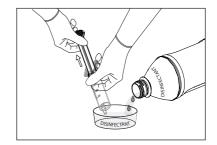
> Press and hold the foot pedal and contemporary start injecting the disinfectant with the syringe until 12 ml of disinfectant are injected
