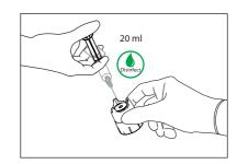
> Use a disposable syringe to aspirate and inject a disinfectant solution (2% (v/v) ID 213 solution, Dürr Dental) into the hose and the male coupling of the Irrigation Circuit Cleaning Kit.
