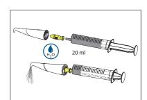
> Rinse the internal channel of the scaler handpiece with tap water for minimum 1 minute (temperature < 35 °C) using a 20 ml disposable syringe.
