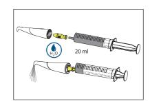
> Rinse the internal channel of the scaler handpiece with deionised water for minimum 1 minute using a 20 ml disposable syringe.
