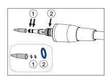
> Use the two small O-rings as assistance in tightening.
