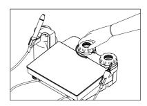
> Pour the Lunos® Prophylaxis Powder Gentle Clean into the container, assuring that the powder level is beneath the angled pressurization duct located inside (the diffuser).
