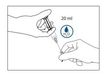
Use a disposable 20 ml syringe to aspirate and inject deionised water for minimum 1 minute into instruments torque wrench hard-to-reach areas (through holes, internal cavities, grooves and crevices). 24
