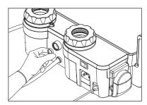
> Re-introduce the filter into its seat and screw the knurled bush back into its housing tightly until it is fully in position.
