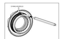
> Clean accurately the o-ring seat from powder residues, by blowing compressed air;
