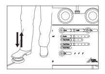
> The "Flush" cycle is performed contemporary on both powder containers. The cycle lasts about 40 seconds. Once it has ended, the touch surface is enabled again, and displays the last setting used.
