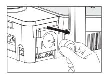
> Connect the new peristaltic pump (REF 2044100054) to its seat until a "click" sound is heard and then connect the two pump tubings to their respective
