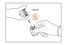
> Use a disposable syringe to aspirate and inject a cleaning solution (2% (v/v) ID 213 solution, Dürr Dental) into the hose and the male coupling of the Irrigation Circuit Cleaning Kit.
