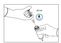
> Use a disposable 20 ml syringe to aspirate and inject deionised water for minimum 1 minute into Lunos® scaler instrument's lumen (internal channel).
