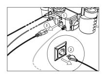
> Disconnect the quick-coupling connector of the external water supply from the device;
