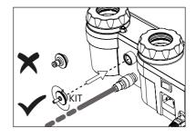
> If it has been previously disconnected (for example for cleaning), connect the hose supplied with the kit to the male water connection:
