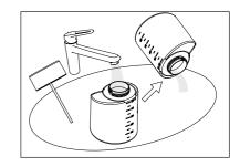
> Fill the water tank with 60 ml of disinfectant (Vector/RinsEndo Disinfection, Dürr Dental). Close the cap of the water tank.
