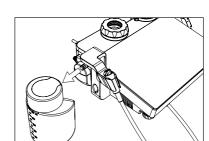
> Unscrew the cap from the water tank and empty it;
